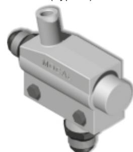
**Type I** For the Rover, Buick, Oldsmobile, V8 where space can be very limited we can supply a replacement oil pump cover with outlets for a remote filter plus oil cooler if required.
