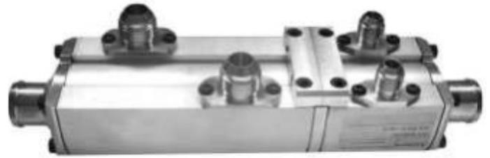
A combined unit for engine & gearbox or gearbox & differential cooling. Available with Male JIC 6, JIC 8, JIC 10, JIC 12, JIC 16 and female M26x1,5 oil connections. Male 28mm, 32mm, 35mm, 38mm, 45mm and 50mm water connections.
