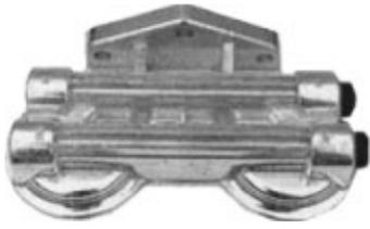
RFH5 takes 2 filters in parallel with 3/4UNF thread, feed and return from either side, 1/2NPTF ports blanking plugs included.
