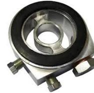
Where there is no suitable block tapping, we have a thin sandwich with 2 x 1/8 NPTF & 1 x 3/8BSP tappings. Made from billet aluminium, supplied with 3 Plugs and extension screw. This will fit cars with a spin on filter, see fitting chart on page 20, SP1 range.
