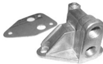
**Type H** Some engines have a cover plate, which may be removed and replaced with a special take off.
