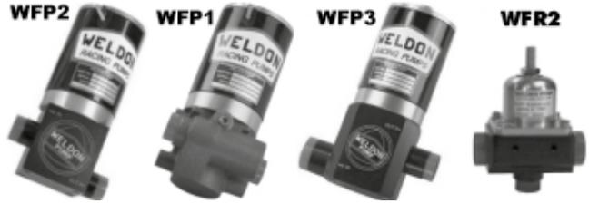
The finest fuel pumps for super high performance with 13 different pumps for engines making 600 to 2400 horse power, we stock 3. Billet aluminium bodies with steel/bronze internals, breakaway motor to pump coupling prevents damage from fuel contamination. No internal filters fitted. Use with regulator except WFP1 which has internal valve and cast body. The regulator has 2 x 1/8NPTF ports for gauge and boost sensor.
