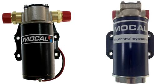
Hardened bronze gear pump. Brass body 12 volt motor. Weight 3lbs. Flows up to 150 gph (UK) 680 litres ph of oil pressure up to 50psi. Max temp 175°C. Current draw 6 to 8 amps. Rubber mounted.
