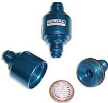
The two part threaded anodised aluminium housing in standard blue, black, red or silver. Removable stainless steel filter, which can be cleaned. Choice of 15, 40 or 120 micron mesh. Essential on fuel systems to protect carburettor and fuel injection pumps. Can be supplied in 2 different halves, e.g. to join -6 to -8 hose. Negligible pressure drop when clean but must be inspected regularly.
