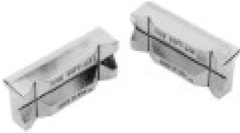
**Construction.** Aluminium die casting with angled pockets to hold any size hexagon and horizontal pocket to hold all sizes of hose. Cast in magnets hold jaws firmly to vice. **Application.** Holds anodised fittings during assembly minimising marking the finish and allows hose to be held firmly during cutting operation.
