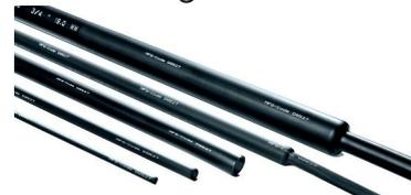
Black high grade PVC, minimum shrink temperature 130°C, shrink ratio is 2:1.
