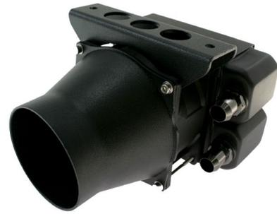
A small and light hot water based heater designed for race and rally cars. These work with one or two universal defrost vents which feed the windscreen. A complete solution for the heater with hose and, fluids, weighs under 2kg. The heater matrix can be mounted with the hose fittings facing towards or away from the 2.5" outlet.
