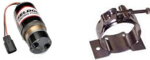
A sliding vane pump built to close tolerance aerospace standards. 14 volt motor. Weight 1.4kg/3lbs. Ports are -6JIC (9/16x 18) female. The pump body is machined from billet aluminium, rotating parts are heat treated high speed steel in precision bearings. Adjustable cam ring for varying pressure/flow. Built in pressure relief valve. Performance. Flow 24gph(UK)/109litres ph of oil at 150°C. Pressure 0-60psi/0-4bar. Temperature for constant use up to 150°C. Max current draw 5.5 amps.
