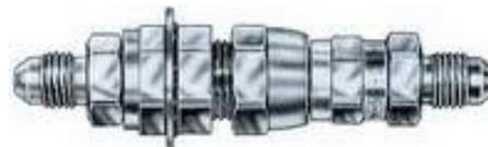
Construction. An Aeroquip threaded steel coupling with provision for bulkhead mounting. Compact and lightweight with very little air inclusion (0.1cc). Overall length 3.52" connected. Application. The finest low cost connection for brake & clutch use. Has EPR seals.
