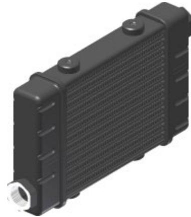
This has a smaller front of 40mm as opposed to the 50mm of the Mocal and STD coolers. Pressure drop will be higher, they are suited for most oil cooling applications but only the 14 row height should be considered for the higher flows found in engine cooling installations. These tube and fin coolers are "Nocoloc" brazed and have a black epoxy finish.
