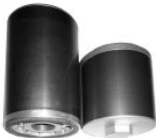
Billet aluminium bodies in two lengths 4.25" & 6.25" overall x 3" width with threads to fit all popular engines, see chart page 20, to take CM's synthetic fibre 8 micron filter(road) or stainless steel 40micron filter (race). Cleaning of steel filters as XRP.
