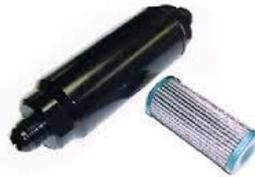
Low restriction oil filter, 240 micron, designed to protect electric pumps used in transmission, differential or turbo charger installations from damage to gears or soft diaphragms. Body is black anodised aluminium and the element is cleanable wire mesh. Dimensions are 160mm long x 45mm diameter.
