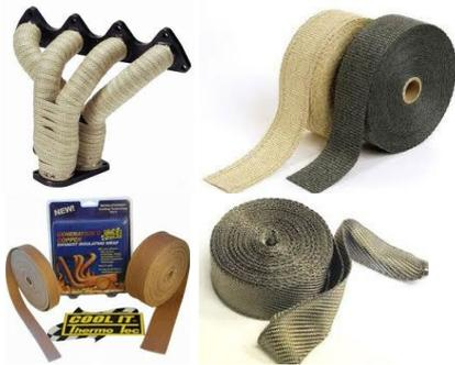
Application. It is widely claimed that insulating the exhaust manifold pipes will produce more horsepower, it will certainly reduce under bonnet temperatures with consequent benefits. Daily use may lead to more rapid corrosion of thin section manifolds. Secure with stainless steel cable/hose ties.
