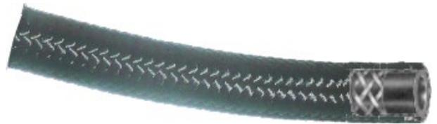
A high performance racing hose compatible with Aeroquip and similar reusable fittings. CPE neoprene tube, Stainless steel inner tube and black braided nylon outer. Resistant to oils, fuels, coolant and alcohols. Temperature range -49°C to + 149°C.
