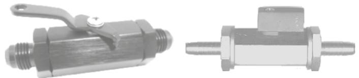
Use for fuel shut off and air jack control. Stainless steel ball valve in teflon seating. Steel body has Nylon handle, Aluminium body has Aluminium handle.
