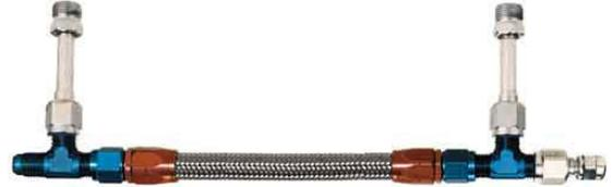
Assembly features a capped -4JIC male to facilitate fitting of a fuel gauge, if smaller bore required use an adapter -3JIC male/female Part No MFA1-3-6.
