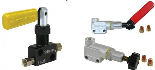
Place in any hydraulic circuit to reduce pressure, maximum reduction 57%. Normally positioned in line to rear brakes, but can be positioned anywhere to produce weird and wonderful effects e.g. on inside front wheel on oval tracks. Aluminium and steel construction. Available with handle giving 7 positive click settings or knob to allow even finer adjustment. Weight 8 oz.
