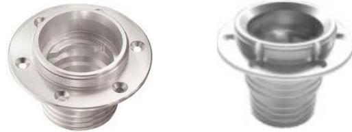
One piece threaded flange and funnel combined, designed to allow for fitment to exterior bodywork and connecting via a hose to a remote tank. They are machined from billet aluminium, polished and then anodised silver or chrome plated. Will take 2.25 (57mm) and 2 (51mm) hoses. Secondary locking filler caps (LIK1) and lead free flaps (LFF1).can be fitted.
