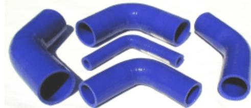
Blue, red or black silicone rubber with smooth wipe down finish. Temperature range -50°C to 250°C. Specials available to order include longer legs, reducing straights and elbows, wire reinforcing, Use for engine coolant hoses, turbo Charger and supercharger hoses, heating and ventilating ducts where increased hose life and resistance to high under bonnet temperatures are required. Compatible with hose joiners on previous page. Please ask for colour and size you want.
