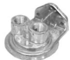
RFH3 takes filter with 3/4UNF thread. Left entry RFH3A has 1/2BSP ports, Right entry RFH3B has 1/2NPTF. 80 & 98mm diameter filters can be accommodated. RFH3A has bosses that may be tapped for pressure/temperature take offs.
