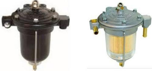
As pressure regulator but with filter, Highflow has aluminium bowl and washable metal filter and 1/8NPTF tapping for pressure gauge take off. The others have glass bowls
