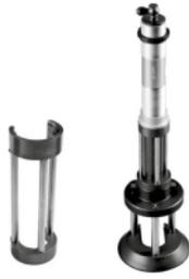
No work under the car should take place without safety props in place, in case of accidental release. The car lifter may be used in place of safety prop and used to provide extra height under the car. To use: Raise car, insert lifter, lower car, insert bar in lifter, raise car.
