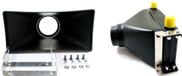
High quality oil cooling air ducts have been specifically designed to mount quickly and easily to 13, 16 or 19 row Mocal or Setrab type oil coolers. Supplied with laser cut aluminium mounting brackets and all fittings. The main body is formed from HDPE. Stepped inlet to accommodate two sizes of ducting 63/76mm on 13 & 16 row. 19 row duct designed with double inlet 76/63mm. Oil cooler not included.
