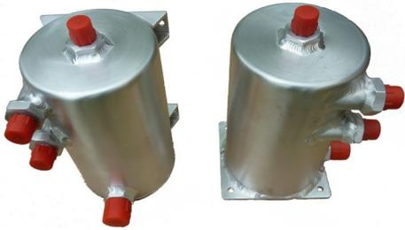
Mainly used with fuel injected engines, these pots act as a surge free fuel reservoir, de-aerator and if mounted in a suitable place, a cooler. Fuel from the tank is fed to the swirl pot by a low pressure pump then by high pressure pump from the pot to the injectors, unused fuel is returned to the pot then to the tank. The three upper connections are -6JIC and the lower connection (to high pressure pump) is -10JIC. Height is 160mm, diameter is 102mm.
