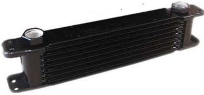
An aluminium pressed plate oil cooler constructed along similar lines to the Mocal and Setrab cooler but with only 37mm depth. The top and bottom plates are not fluid carrying. Despite its smaller depth, performance is very competitive with Mocal and Setrab coolers of comparable frontal area, although oil pressure drops are higher. Supplied with 7/8 x 14 (-10) UNF female threads. For adapters see page 51 onwards. Very nicely finished in glossy black.
