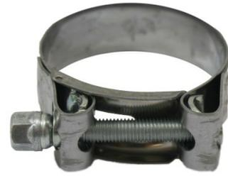
The Supra W4 (pro) clamp from Mikalor is made of 304 marine grade stainless steel throughout. These wide band T-Bolt clamps are excellent for use with silicon hose, especially high-pressure applications.
