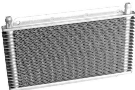
The PWR range of 19mm deep coolers is of aluminium pressed plate construction, they are configured to suit cooling systems powered by electric remote pumps with their lower oil flows than engine driven pumps. Compared to our range of 50mm deep coolers their narrower oil passages offer higher oil flow resistance but this is of
