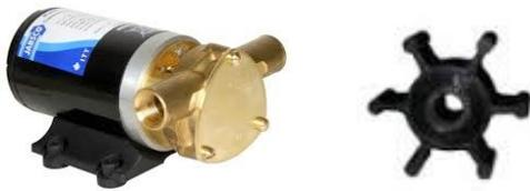
Construction. 12 or 24 volt electric motor with brass pump housing and neoprene impeller, although rated for modest temperatures has proved satisfactory for elevated temperatures encountered. We recommend that an extra impellor housing gasket be fitted for temperatures above 90°C. Weight 3kg. Ports are ½ BSP. These pumps were widely used in the early '60s so good for historic.
