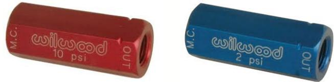
These in-line pressure valves retain a minimum brake line pressure to help eliminate excessive pedal travel. Use 2psi for discs and 10psi for drums. Made from billet aluminium. Size 40mm x 16mm
