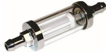
Construction. Chrome plated steel end caps, glass housing with 40 micron plastic filter which may be removed for cleaning. Application. Use on carburettor systems, not above 10psi.
