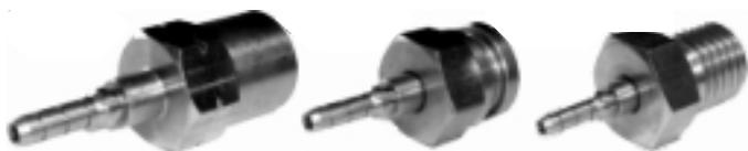
Non swivel, Threaded takes M16x2.0 nut. Circlip uses original snap clip. Direct fitting onto metal brake pipes with male nuts.
