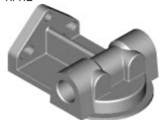
RFH1 takes filter with 3/4UNF thread. A compact design which will require a spacer if a filter larger than 80mm diameter is mounted against a flat surface. Provision can be made to take a capillary type temperature gauge sender or pressure gauge tapping. Available in either flow direction. Has 1/2BSP female ports
