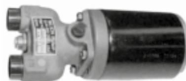
Construction is similar to above but more suited to lubricating under pressure. Adjustable pressure relief valve. Flow 17 gals/75 litres per hour @ 25psi
