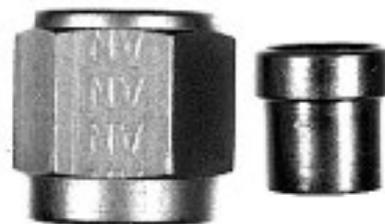
Aeroquip two part blue anodised aluminium female JIC fitting for attachment to Bundy, Kunifer, steel or aluminium tube, requires the use of a flaring tool.
