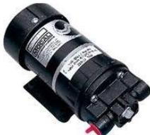
A diaphragm pump, has integral cooling fan, 12 volt motor. Weight 1.5kg. Ports are 3/8NPTF and may be rotated in 90° increments to simplify plumbing. The pump body is made of lightweight nylon, care must be taken when tightening tapered adapters not to over tighten and crack housing.
