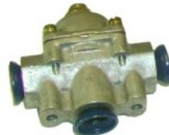
It has a painted aluminium body with three 3/8 NPTF female ports, one inlet and two outlets one of which may be blanked if not required or used as a tapping for a fuel pressure gauge / indicator.
