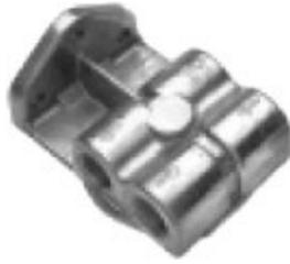
RFH6 takes filter with 3/4UNF thread, feed and return from either side, 1/2NPTF ports blanking plugs included.
