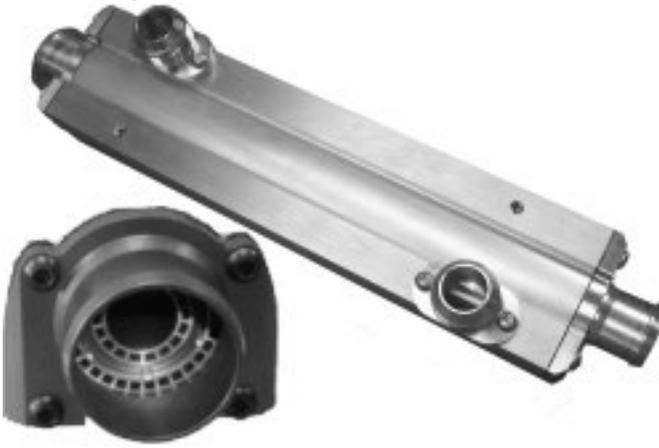
Provides engine oil cooling for more demanding applications. Construction is similar to C43 range except oil outlets are parallel not on opposite sides. Available with twin oil side cores, one fitted inside the other. Heat transfer for the twin core example is almost double the C43-330. Currently available with oil side connections in -8, -10, -12 & -16 SAE 37° (JIC) and waterside to take 28, 32, 35, 38 and 45mm bore hose.
