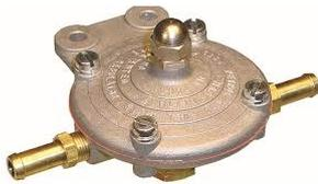
Although much touted as fuel saving gadget, it is a proper fuel pressure regulator for carburettors, set at 2psi but adjustable it should be set up with a pressure gauge in accordance with carburettor manufacturers' recommendation. Incoming pressure not above 10psi. The body is pressure die cast aluminium with neoprene membrane suitable for most fuels except methanol, adjustment 1.5-5psi. Inlet & outlet ports are tapped. 1/8 NPTF, supplied with 5/16" straight connectors
