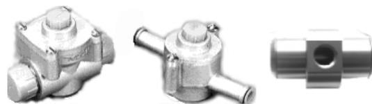
A range of adapters to take all types of capillary gauge, they are designed to be fitted into oil or water hoses. Oil hose adapters are 2 part aluminium die castings with an O ring seal. Hose connections are male push on, JIC, BSP or female NPTF. Water hose adapters are machined from billet and blue anodised. Also see page 21 "Take off plates with temperature gauge tappings"
