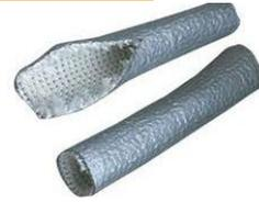
This heat resistant sleeve is lighter and less bulky than Aeroquip firesleeve is made from woven fiberglass with a silver silicon rubber coating Temp range -40°C to 220°C
