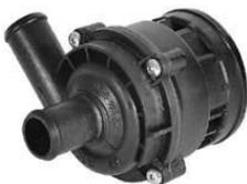
Construction. 12 or 24 volt brushless motor connected to impellor in nylon housing via magnetic coupling. Overall length 97mm, Overall diameter 69mm, weight 0.25kg., has 3/4" push on connections. Performance. 13.3 litres/min at 0.12 Bar (1.7psi), current draw 0.7amp (12v). Temperature range -40 to 135°C. For users of the EWP/1 & 115 this pump can operate on the heater circuit for constant heater supply or in LPG installations requiring a heated manifold.
