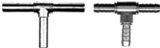
Assemble with swage ferrule, O clamp or worm drive clamp. Suitable for low pressure systems e.g. carburettor feeds, breathers.
