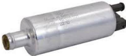
Very small 130mm x 36mm overall weighing 0.5lbs with 15mm inlet and 8mm outlet push on fittings. Flow 40 gph (UK), pressure up to 10psi. Max temperature 170°C. 8 amp rating. Filter on inlet.
