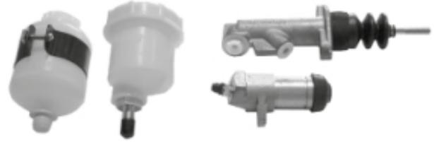
Girling manufactured. Master cylinders have 1.4" stroke with 7/16UNF inlet with concave seating and 3/8UNF outlet with convex seating. The reservoirs either screw directly to master cylinder or may be mounted remotely and fed through a 7mm hose.
