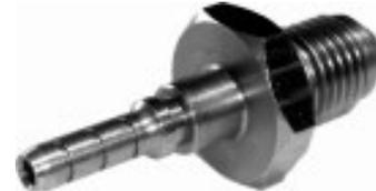
Non swivel, direct fitting into calipers, master and wheel cylinders. Convex & concave seal on bottom of port.
