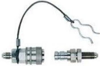
Aeroquip plated mild steel with EPR seals, length connected is 4.10 inches and weight 0.34 lbs. Max operating pressure 3000psi, max temperature 120°C. Allows rapid connection & disconnection of brake & clutch lines with little fluid loss, 0.10cc max, minute air inclusion 0.02 cc max, obviating the need for bleeding. A safety clip-on lanyard is attached to the coupling to prevent accidental disconnection.
