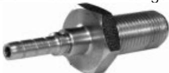
Non swivel, direct fitting into calipers, master and wheel cylinders. Convex & concave seal on bottom of port.
