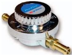
Chromed alloy body with 1/8NPTF female threads, supplied with push on fittings and hose clamps. Can be set from 1-5psi on calibrated dial.
