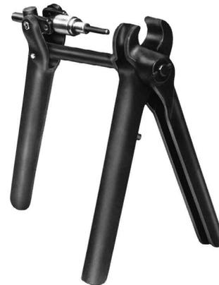
The FT1268 / FBM3632 hand held assembly tool designed for assembly of -4,-6 & -8 straight fittings into push on hose, tool for angled fittings available soon. The hose is held in position by manually operated clamp, and the fitting is positioned on the mandrel assembly lever. The fitting is pushed into the hose by compressing the mandrel assembly lever.
