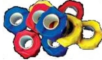
Silicone tape with tear off backing. This specially formulated self-amalgamating tape bonds to itself without any adhesive. Wrap the tape tightly around the substrate, and it will cure to itself without leaving any sticky residue. Slightly triangular in shape, it has a centre line to enable regular overlapping of the tape. Temp range -40°C to 220°C
