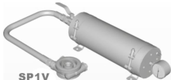
3. For engines with a disposable element filter use a standard take off plate Tee off a loop and fit a one way valve, [see page 58](#) or Accusump check valve ACCUV2, to prevent oil returning through the pump.
