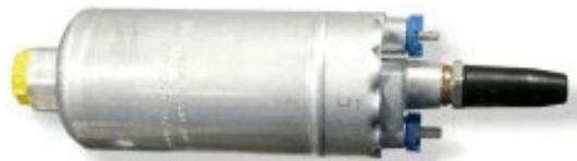
Bosch pumps have steel bodies 168 x 60mm x with M14 x 1.5 or M18x1.5 intake, M12 x 1.5 outlet, pressure 5Bar. Max current 10amps, weight 1kg approx. We can supply a blanking cap to allow a banjo fitting to be fitted to outlet.
