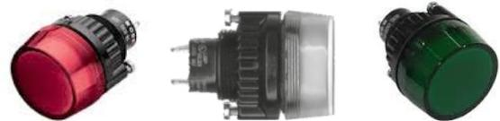
These are of little use if they are not immediately visible, ours are 29mm diameter with a choice of red, yellow, green, blue or clear lens, these have a removable diffuser under the lens which may be titled using dry print lettering. A T5.5 side contact bulb is accessed from the front and is sealed against ingress of dust, oil and water. Weight is 1.5 grams.
